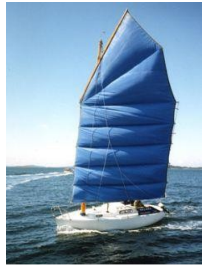
1999, with taller mast and 7 panels.
